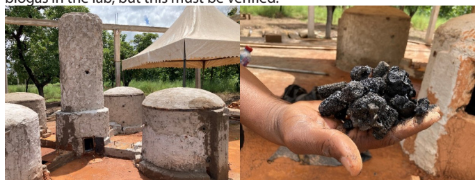
Figure 1 Newly constructed Brazilian kiln with four chambers and common chimney and resulting corn cob biochar in Loagri, Ghana
